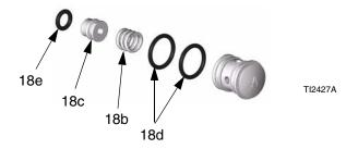
**11.** Liberally lubricate and reinstall side seal cartridges (18).
