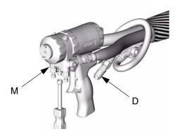
**3.** Unscrew cylinder cap (5). Hold piston stop (28) with wrench and unscrew from safety lock (4). Inspect spring (30) and o-rings (14, 24).
