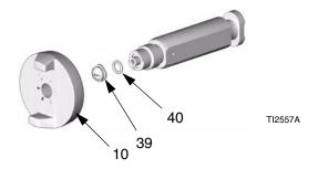
If tip is stuck, pry off with small screwdriver or pull off with pliers. Tip is hardened to resist damage.
