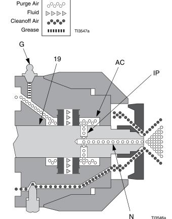
**3.** Remove grease fitting cap. Using grease gun (Y), dispense grease into fitting (G) until grease mist sprays from mix chamber nozzle (N). Do not over-grease; use 2 shots maximum. Do not spray grease mist on sprayed material.
