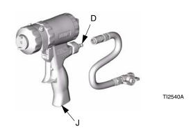
7 Attach fluid manifold. Connect air. Return gun to service.
