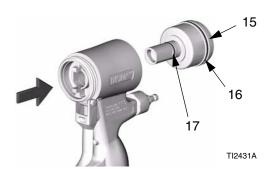
**6.** Liberally lubricate piston o-rings. Reinstall piston. Shaft is keyed for proper assembly. Push firmly to seat piston.
